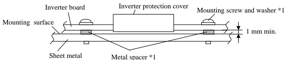
\*1: The conductive material (mounting screw, washer, metal spacer and so on) is allowed to mount within the limits of 2.5mm radius from the center of mounting hole. ☆
