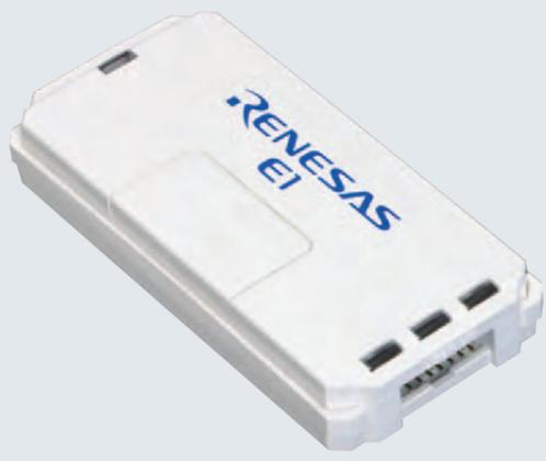
An affordably priced model that doubles as a flash programmer and provides basic debugging functions including on-chip trace.
