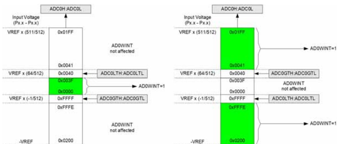
Figure 5.8. ADC Window Compare Example: Right-Justified Differential Data
