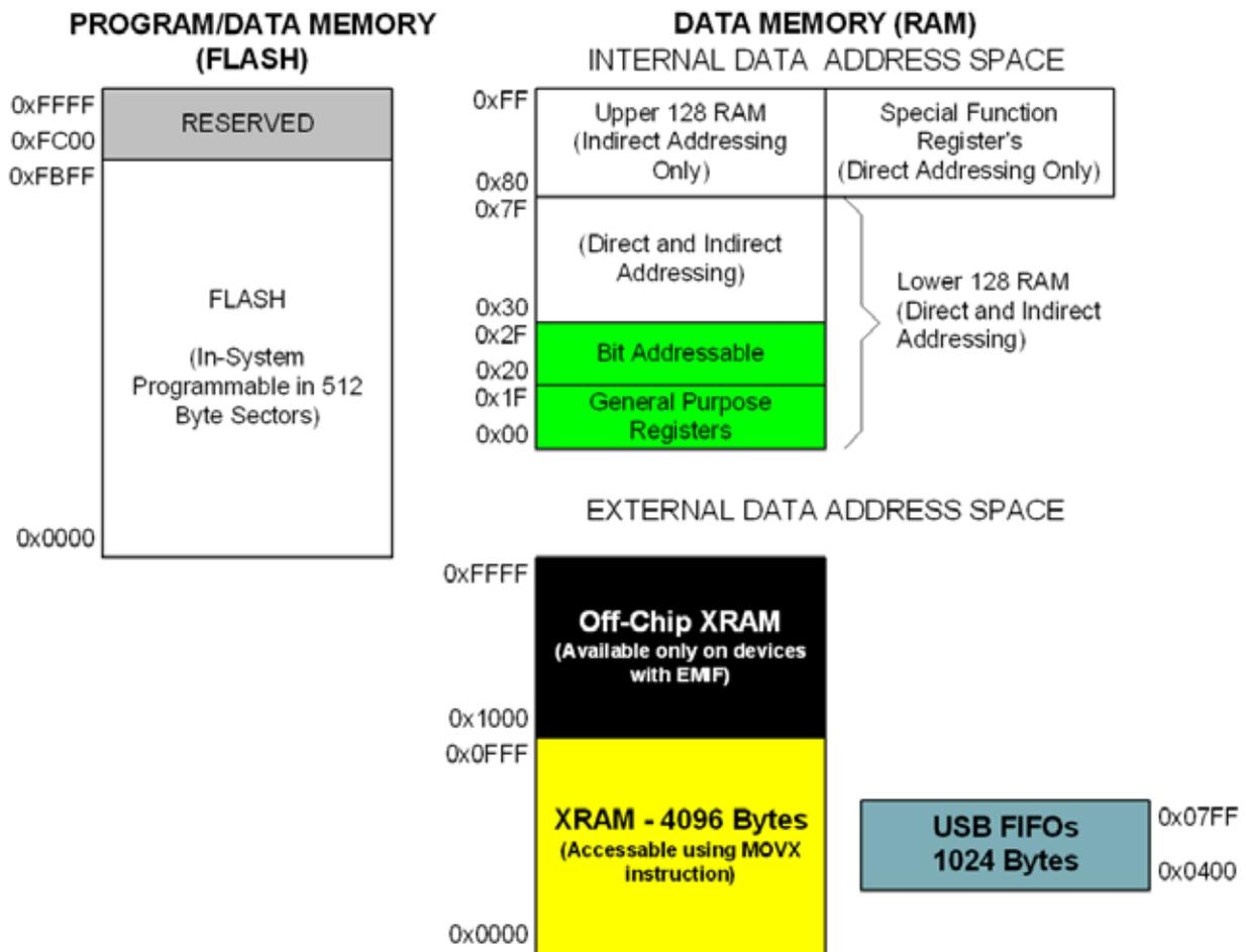
Figure 9.2. On-Chip Memory Map for 64 kB Devices
