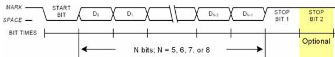
Figure 19.2. UART1 Timing Without Parity or Extra Bit
