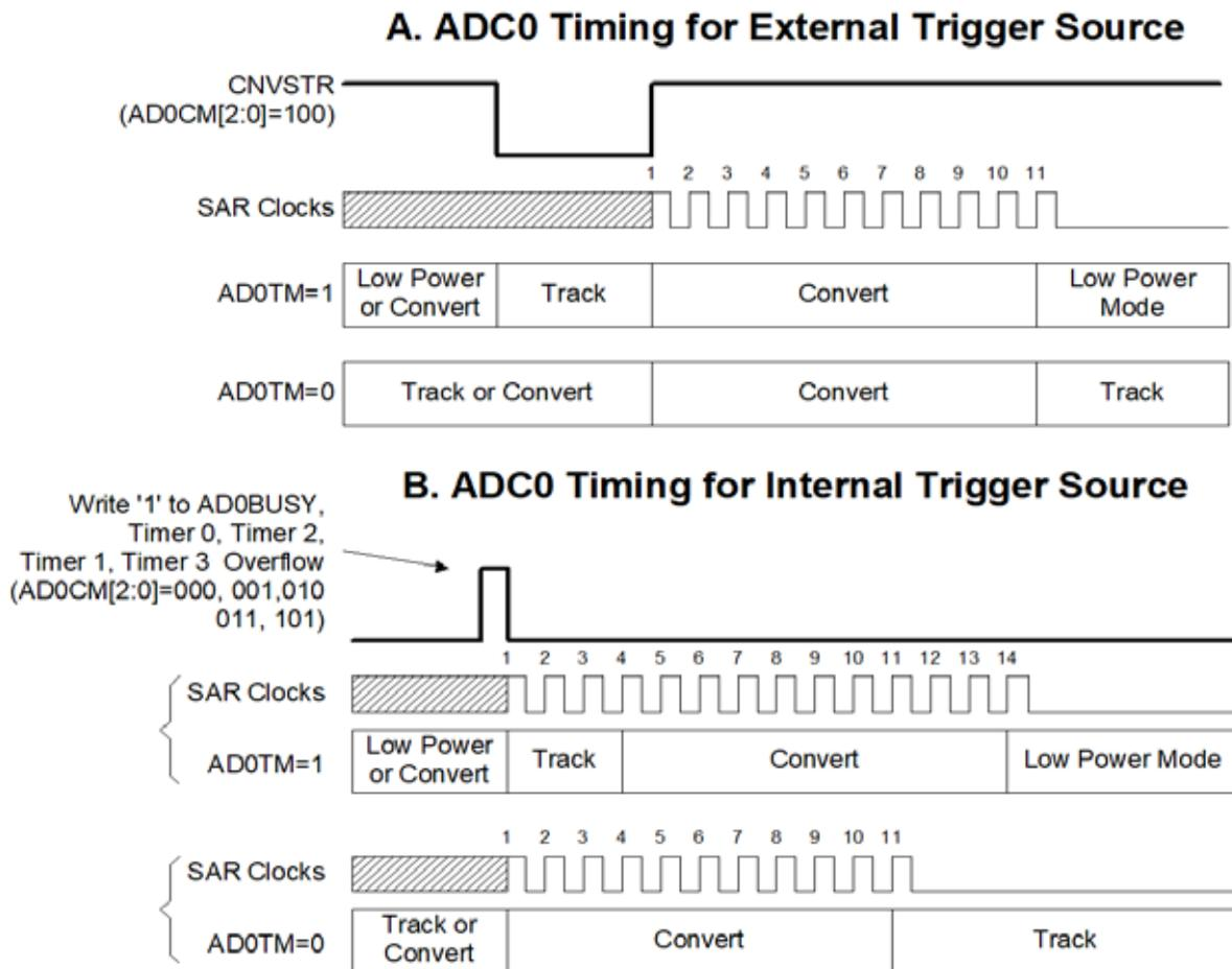
Figure 5.4. 10-Bit ADC Track and Conversion Example Timing
