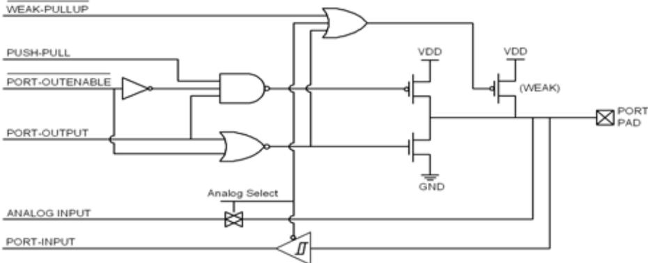
Figure 15.2. Port I/O Cell Block Diagram
