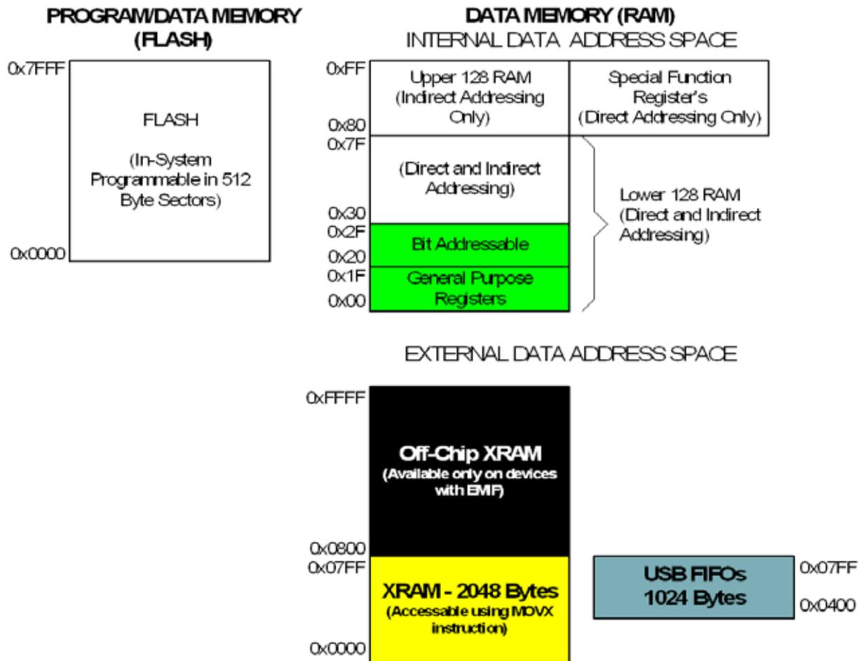
Figure 9.3. On-Chip Memory Map for 32 kB Devices
