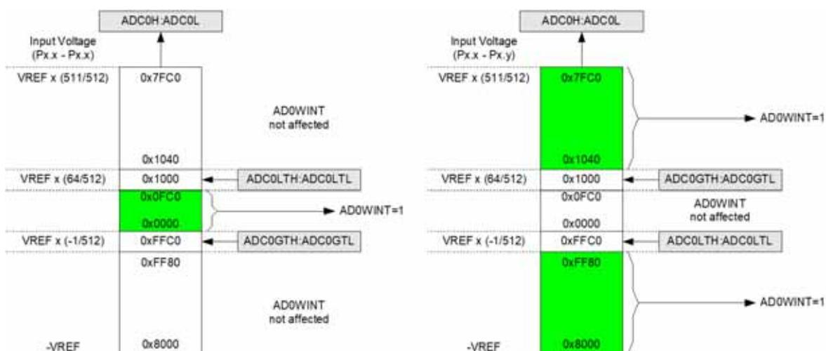
Figure 5.9. ADC Window Compare Example: Left-Justified Differential Data
