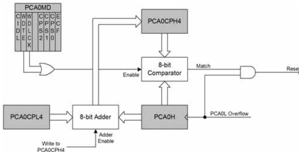
**Figure 22.10. PCA Module 4 with Watchdog Timer Enabled**
