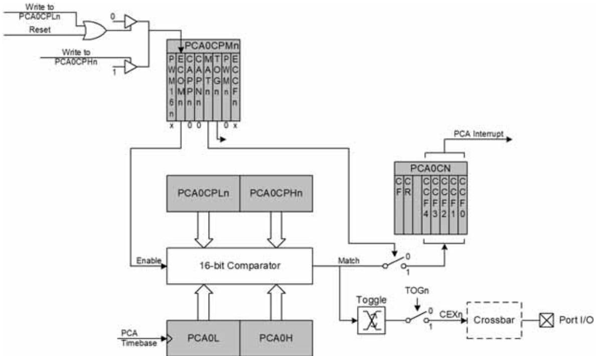
Figure 22.6. PCA High Speed Output Mode Diagram
