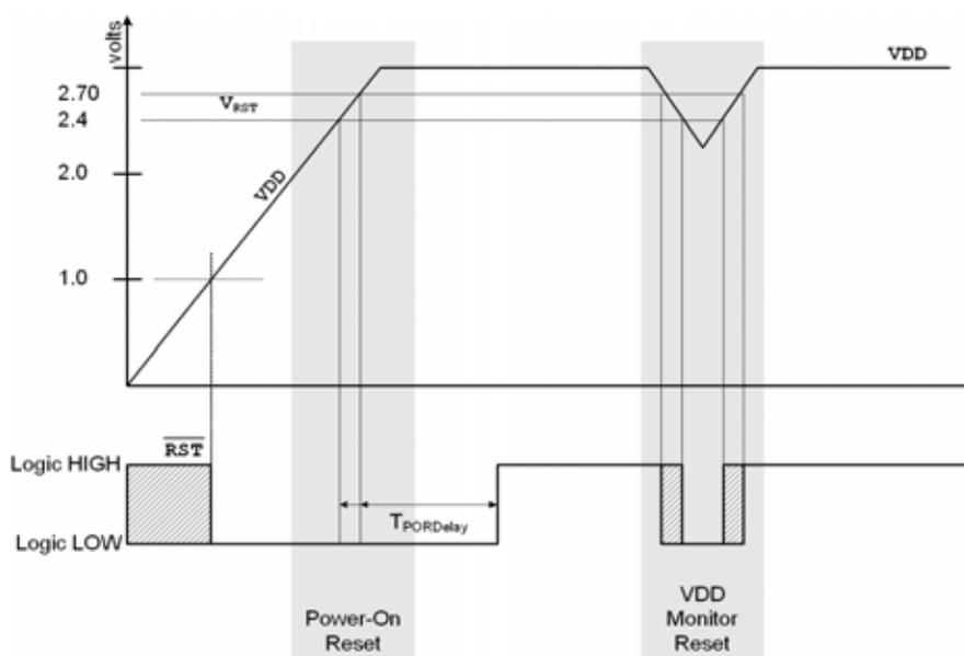
Figure 11.2. Power-On and  $V_{\text{DD}}$  Monitor Reset Timing
