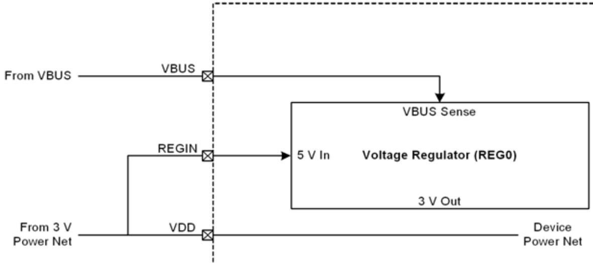
**Figure 8.3. REG0 Configuration: USB Self-Powered, Regulator Disabled**
