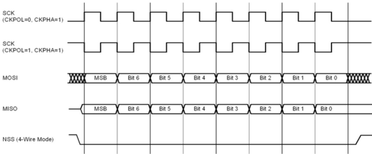
Figure 20.7. Slave Mode Data/Clock Timing (CKPHA = 1)
