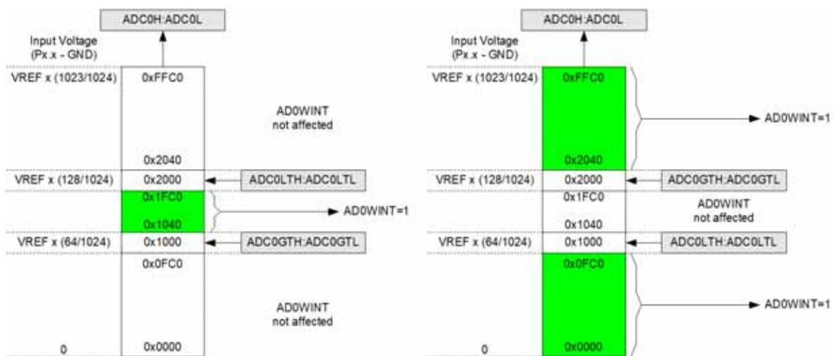
Figure 5.7. ADC Window Compare Example: Left-Justified Single-Ended Data
