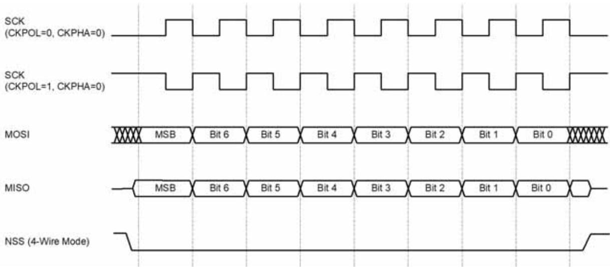
Figure 20.6. Slave Mode Data/Clock Timing (CKPHA = 0)
