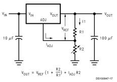
FIGURE 2. Basic Adjustable Regulator
