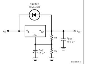
FIGURE 5. Regulator with Protection Diode
