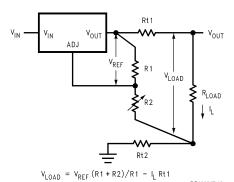
FIGURE 4. Best Load Regulation using Adjustable Output Regulator
